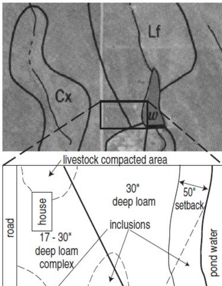
**Figure 1.** Typical soil map of central Kansas and detail of homesite area showing inclusions and local variations.
