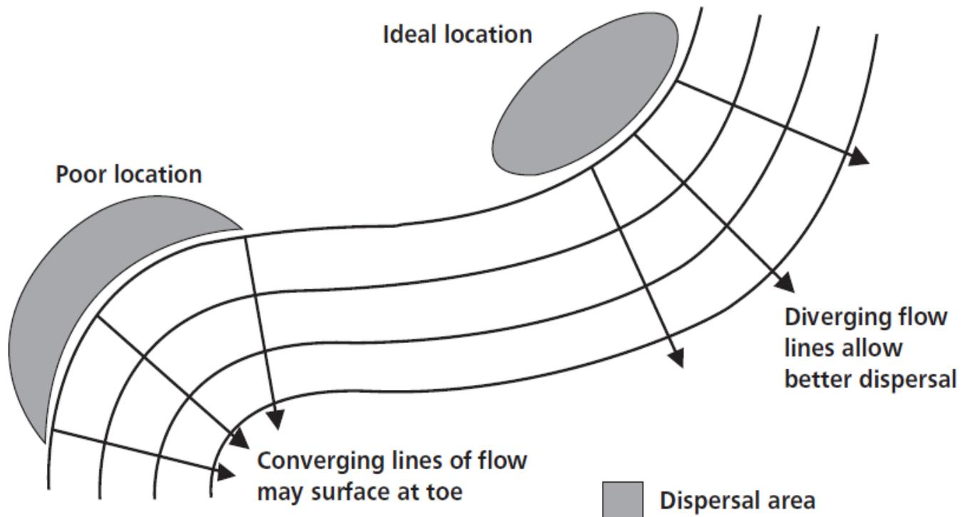
**Figure 3.** Site with complex slope depicts good and poor locations for onsite wastewater systems.
