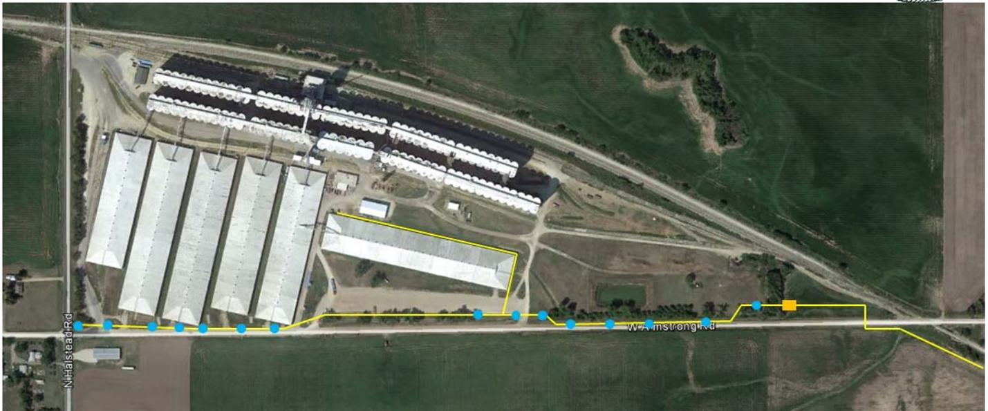
*Fifteen extraction wells (blue dots) pump contaminated groundwater to an air stripper (orange square) for treatment.*
