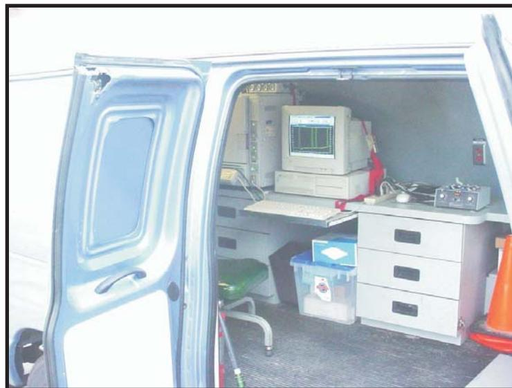
*KDHE Mobile Laboratory being utilized to obtain real-time data during field work at the site.*
