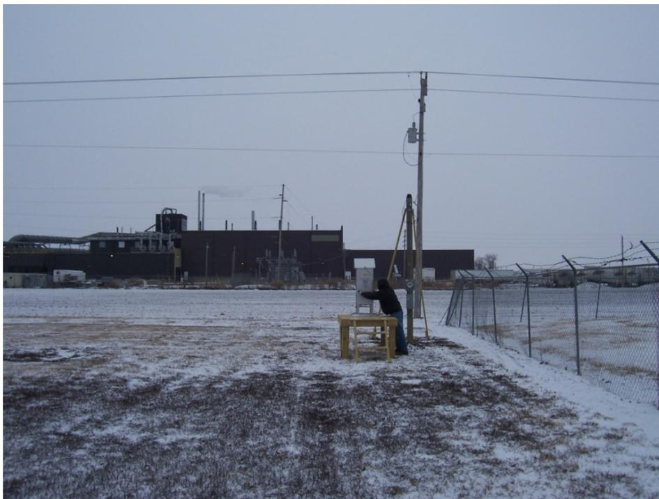
In 2013, KDHE installed a second HiVol TSP sampler at the Exide monitoring site for collocation purposes. Installed next to the existing monitor, the second monitor operates on the same 1-in-6 day sampling schedule as the initial lead monitor. The Salina Exide plant is the only Kansas source that exceeds the 0.5 ton per year point source threshold for the mandatory 2008 Lead NAAQS Nonattainment SIP inventory.
