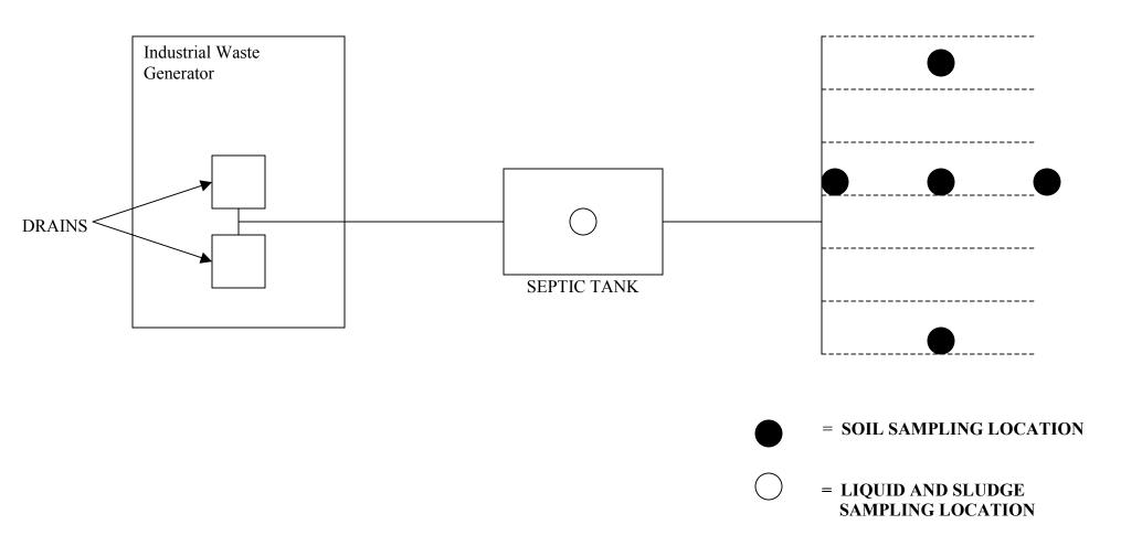
The soil sampling locations shown meet the minimum requirements of the KDHE UIC Program. However, the owner and/or operator is responsible for adequately assessing the extent of any soil or groundwater contamination. This may require additional sampling locations.
