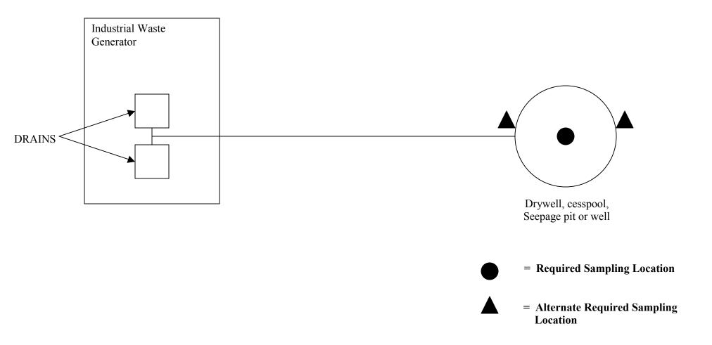
The soil sampling locations shown meet the minimum requirements of the KDHE UIC Program. However, the owner and/or operator is responsible for adequately assessing the extent of any soil or groundwater contamination. This may require additional sampling locations.
