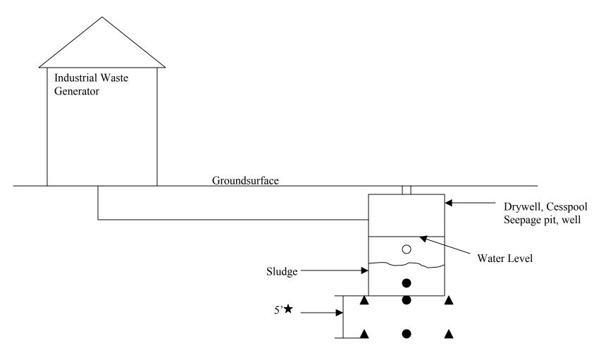
The sampling locations shown meet the minimum requirements of the KDHE UIC program. However, the owner and/or operator is responsible for adequately assessing the extent of any soil or Groundwater contamination.
