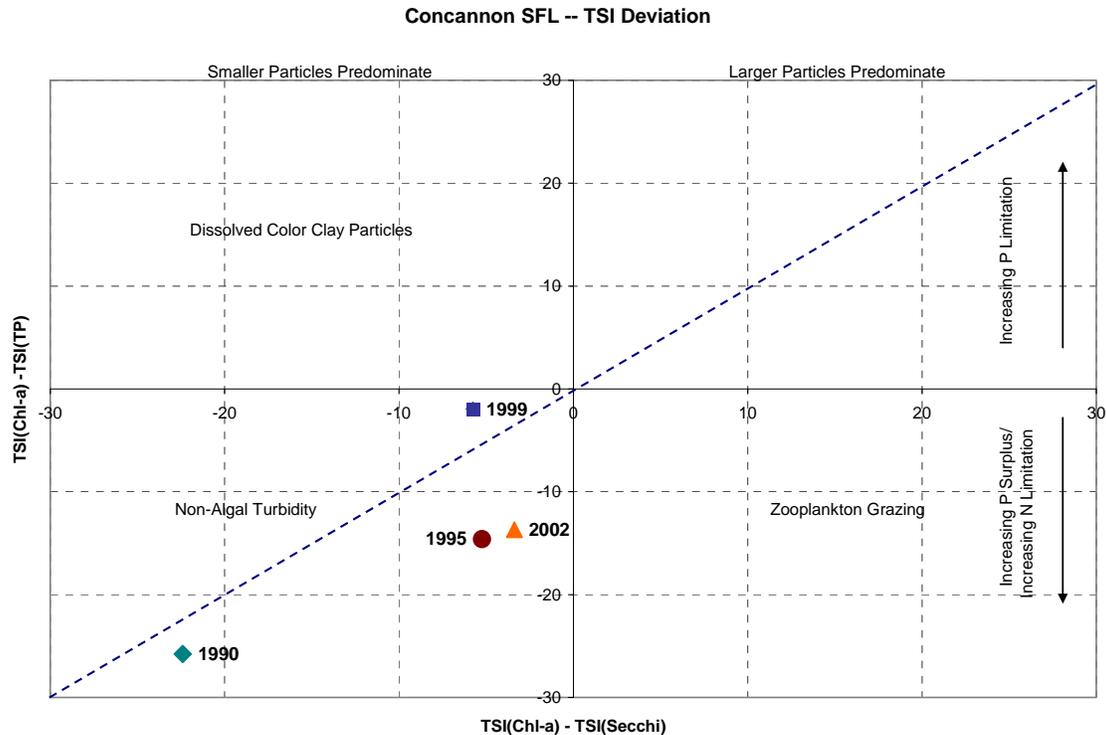
The multivariate TSI comparison chart in Figure 6 indicates non-algal turbidity may be limiting chlorophyll *a* production in Concannon State Fishing Lake. Figure 6 also indicates phosphorus may have been bound to the clay particles during the 1995, 1999 and 2002 samplings while turbidity may have been limiting Chlorophyll *a* production during the 1990 sampling.
